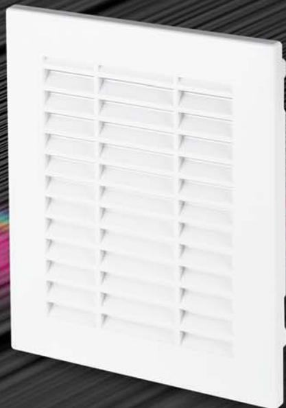
TVZ is a new version of the ventilation grille with louvres. The louvres have been designed to allow closing the grille tightly, and to reduce the air flow completely. Another advantage of the TVZ series grilles is their mounting system. Its main element is spreaders to ensure that the ventilation grille is firmly seated in the mounting hole. The grilles in this series are made of ASA plastic. For specifications, see page 18.
